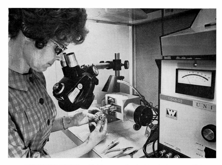
**RESISTANCE-TYPE WELDING** is used by Delores Smith as she works on a Marx generator. Each device has 135 welds and differences in combinations of metals require six or seven weld "schedules" (adjusting the pressure and heat factors).
